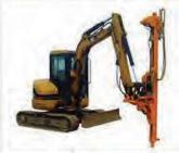
Heavy-duty Feed - Available in an 8' or 12' length, the MDA Drill features a heavy duty feed originally designed for underground hard rock mining. Standard on the drill is a feed brake, football style lubricator, a robust drive system and proven hydraulic components
