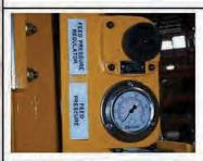
Adjustable Feed Pressure -The MacLean MDA Drill Feed features an adjustable feed pressure. Just set the pressure for the rock conditions and begin drilling!
