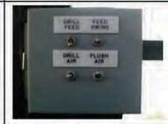
In Cab Controls - The MDA Drill is controlled from within the operator cab, in addition to the standard feed mounted controls. With an enclosed cab the operator is free from any dust, debris and noise. Simply engage the flushing air, turn on the drill, and advance the feed; and you are drilling!
