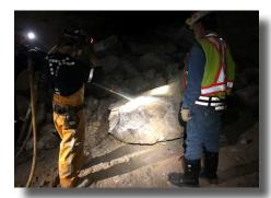
were there when it was formed, understanding the layering, weaknesses and best methods to release it from the earth. With Nxburst™ this type of understanding is even more crucial. With no shockwave and detonation, there needs to be a greater understanding of exactly how much work each cartridge is going to be required to do. With an understanding of the rock to be blasted, its graining, layers and weaknesses, Nxburst™ can be used with great precision to exploit the
