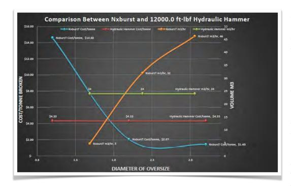
Sometimes a hydraulic hammer make perfect sense. You may already own the excavator, own the hydraulic hammer so why not use it. If you have a small concrete removal job or a few pieces of over-size rock to break then a hammer works well. As soon as you have any significant volumes or material to remove however it can be incredibly time consuming. A hammer is very noisy and can actually cause significant vibration
