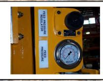
Adjustable Feed Pressure -The MacLean MDA Drill Feed features an adjustable feed pressure. Just set the pressure for the rock conditions and
