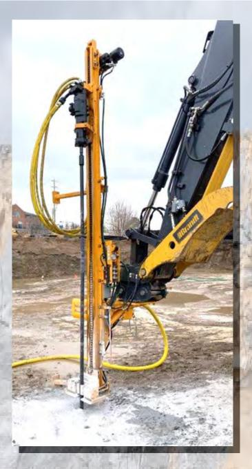
Heavy-duty Feed - The MDA Drill features a heavy duty feed originally designed for underground hard rock mining. Standard on the drill is a feed brake, on-board lubricator, a robust drive system and proven hydraulic components
