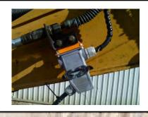
Quick Connect - Should it be needed, the MDA Drill is fully removable with two pins, two hydraulic quick disconnects, and 1 electrical quick disconnect
