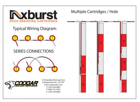
Having held our first training sessions of the year and with the construction season knocking on the door, now is a good time to go back to some basic good practices when using Nxburst™ cartridges. As shown in the diagram, when using electrical Nxburst™ cartridges, single series circuits are a must. This type of circuit wiring can be easily described as in one end and out the other.
